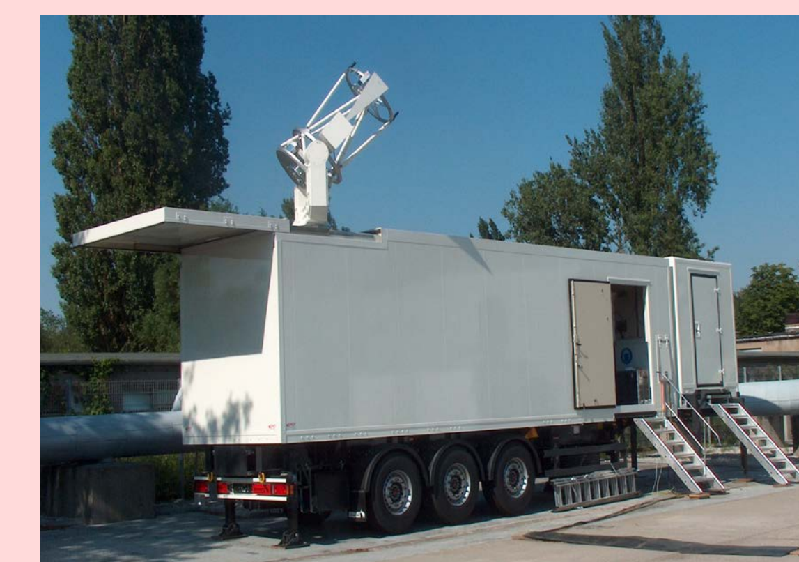
Fig.6. IPM water-vapor DIAL system mounted in mobile trailer. The transmitter is operating at 820 nm and delivers an average power of 6 W. The receiver consists of a 3D 80-cm scanner with an APD photodetector unit.
