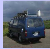
Mobile platform on which the X-Band radar is mounted
