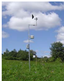
Fig.1: One of the Hobo weather stations operated with a 3m wind mast including the T/RH-sensor and pressure-sensor. The rain gauge is mounted on a separate pole.
